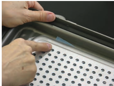
Container filter media must be inspected for integrity and proper placement.
