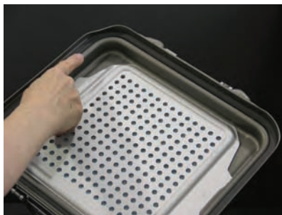
Container lids must be inspected for dents and chips.
