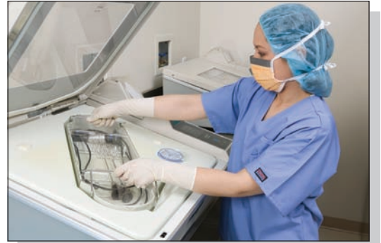
Peracetic acid-based low-temperature liquid sterile processing
