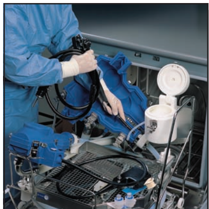
High-level disinfection in an automated endoscope reprocessor
