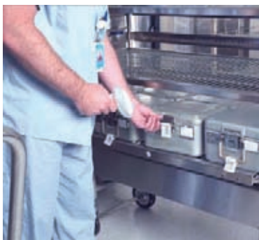
Figure 4: As items are scanned into a sterilizer load, information can be provided about weight, mass and density aspects of load configuration, compatibility of items to sterilant, and the necessity of extended cycle alerts, if required.
